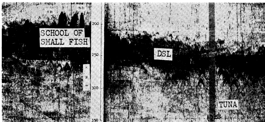
Fig. 11. The echo-trace of tuna appearing at the similar zone to that of migratory scattering layer. (1964, 7. 12, noon, 29°N, 127°E, Nagasaki-Maru, P.D.R. 14 kc).
