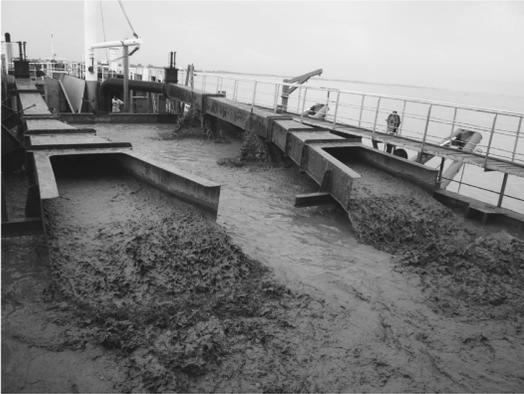
Fig. 3. Dredging ship and bottom material (mixture of sand and water) taken from Inner Bar (16° 45.817'N and 96°11.945'E) on 16<sup>th</sup> September 2010.
