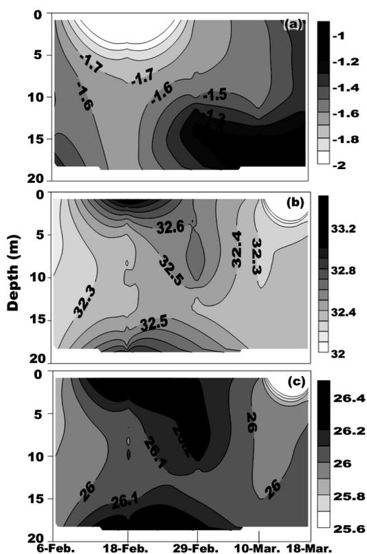
**Fig. 2** Time courses in vertical section of temperature (a:  $^{\circ}\text{C}$ ), salinity (b) and density (c: sigma-T) in the water column observed during the ice-covered period from February 6 to March 18, 2008, at the fixed station in Lagoon Notoro-ko on the Okhotsk Sea coast of Hokkaido, Japan. The bottom depth was about 20 m.
