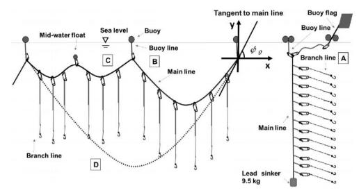
Fig. 1 Vertical and horizontal longline at RT/V Seiyo Maru.
