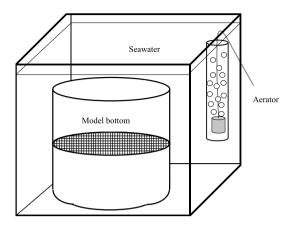
Fig. 1. Experimental model of biofilm formation at the aquatic benthic boundary. The model bottom (nylon mesh, 50 μm) was affixed in a transparent acrylic vessel (diameter, 9.5 cm; height, 15 cm) with a closed bottom and an open mouth. The acrylic vessel was submerged in a glass chamber of dimensions 18 cm (D) × 30 cm (W) × 24 cm (H).
