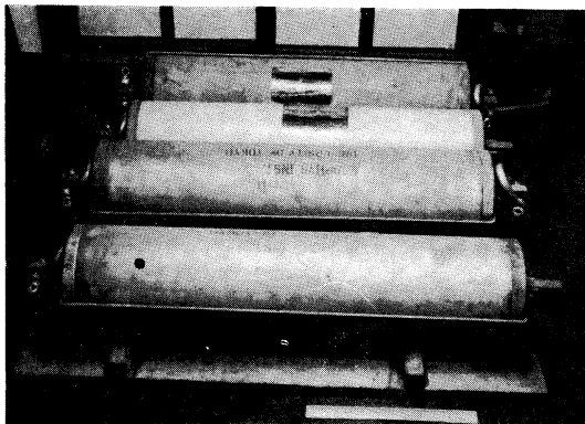
Fig. 3. Pressure vessels. Their dimensions are 18 cm in diameter and 81 cm in length. The third vessel is made of FRP.
